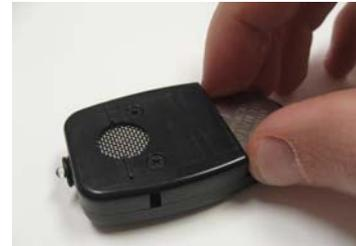
6. Remove old battery. Wait 10 seconds before inserting new one.
