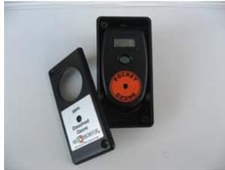
2. After removing screws, remove face-plate, exposing the instrument inside.
