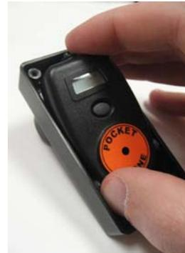
3. Put aside face-plate and remove the instrument from the cavity inside.
