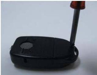
4. Lay the instrument face-down, and remove the screw from the battery cover. Put screw aside (don't lose it!).
