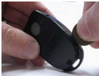
5. Use coin to remove battery cover. Turn coin *clockwise*. Battery cover will pop off.
