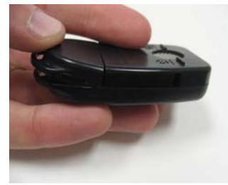
9. Replace cover, as shown. Cover will snap into place. Replace screw. Place instrument back into the adapter case, and replace 2 screws on face-plate.
